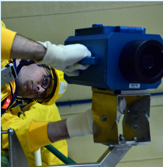
An IAEA safeguards inspector setting up a surveillance camera at a nuclear facility.
